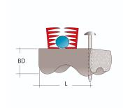
The mounting supo is used to fix the mounting reinforcement. The mounting supo is nailed to the formwork using the factory-fitted aluminum nail. The reinforcement bar (Ø 3-18 mm) is simply inserted into the plastic clip. This enables the reinforcement to be set up quickly. Thanks to the specially designed shape of the clip, the Supo clamps optimally to the reinforcing steel.
