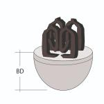
The poured concrete spacer has a round contact surface. The double clamp clamps well to the reinforcing steel. The spacer can be installed on both vertical and horizontal reinforcement. Installation is possible on reinforcement  $\emptyset$  6-16 mm.
