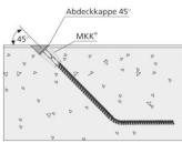
Made from weldable and bendable BETOMAX® tie rods 15, 20 and 26.5 For anchoring supports, for single-sided formwork Installed in first concreting section, in floor slab Can be extended with threaded connecting sleeve and MKK®
