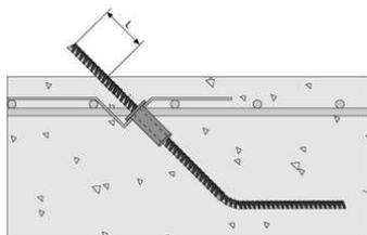
Steel strip and plastic sleeve for anchoring aids for single-sides wall formwork.
