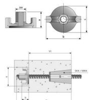
Casting, for one-sided anchoring. Max. load depends on the concrete quality and anchoring depth (Vt). Compatible with Uni 15.
