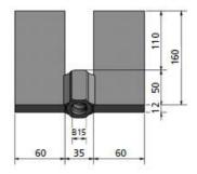
For welding at inclinated areas, e.g. sheet pile walls.
