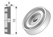
For sealing the MKK® on rough surfaces with angle compensation up to  $3^{\circ}$ .
