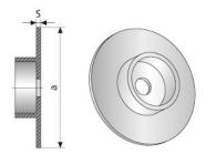
Prevents penetration of concrete into the MKK®.
