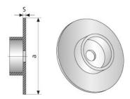
Prevents penetration of concrete into the MKK®.
