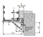
For narrow decks on ramps or wing walls and retaining walls.
