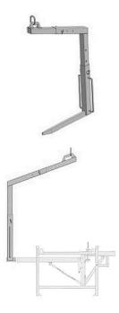
Crane mount to help assemble the pre-assembled cornice brackets.
