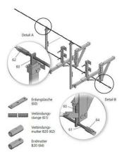
For grounding the canopy framework over electrified railroad lines. Approval of the DB available.
