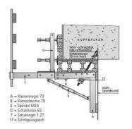
With the BETOMAX® sheet piling bracket 2000/70-s it is possible to produce head beams on sheet piling profiles safely and efficiently. All the advantages of the BETOMAX® cornice bracket 2000 in terms of adjustment options and safety devices (e.g. walkway with railing posts) can be used.
