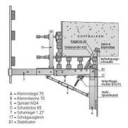
With the BETOMAX® sheet pile bracket 2000/70-k it is possible to produce head beams on sheet pile profiles safely and efficiently. All the advantages of the BETOMAX® cornice bracket 2000 in terms of adjustment options and safety devices (e.g. walkway with railing posts) can be used.
