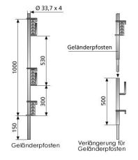
In accordance with the safety rules for side protection and roof protection walls as fall protection during construction work (BG-I 807 from October 2002).
