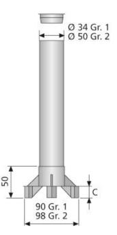
Railing post holder for holding the BETOMAX® railing post in the area of ceiling edges. Installation on the formwork in the edge area of ceilings (built-in part remains in the concrete).
