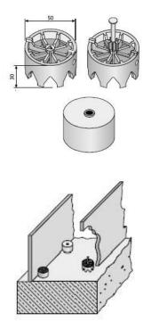
For adjusting the formwork on the underlying component.
