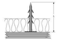
BETOMAX® insulation board holder made of plastic.
